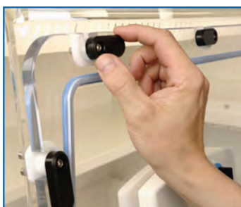
Easily removable front for equipment and bulk sample transfer and thorough cleaning
