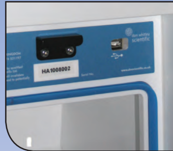
Convenient USB memory stick download of stored environmental parameters
