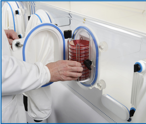
The glove ports can be used as mini-airlocks.
